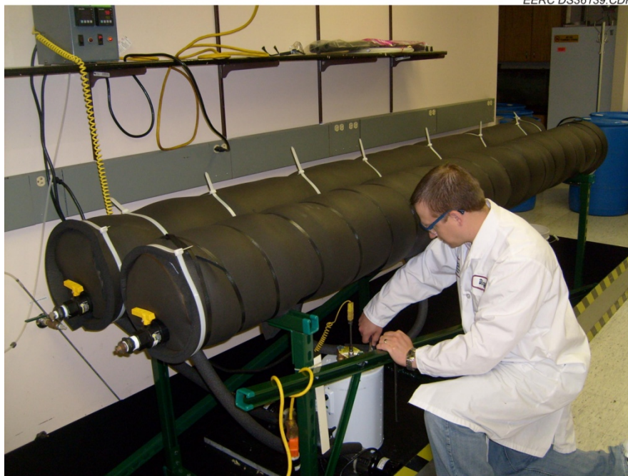
Figure 23. Closed-cell foam insulated digesters.
