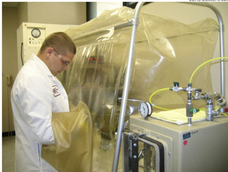
Figure 1. EERC researchers prepare biological experiments in an anaerobic glove box.
